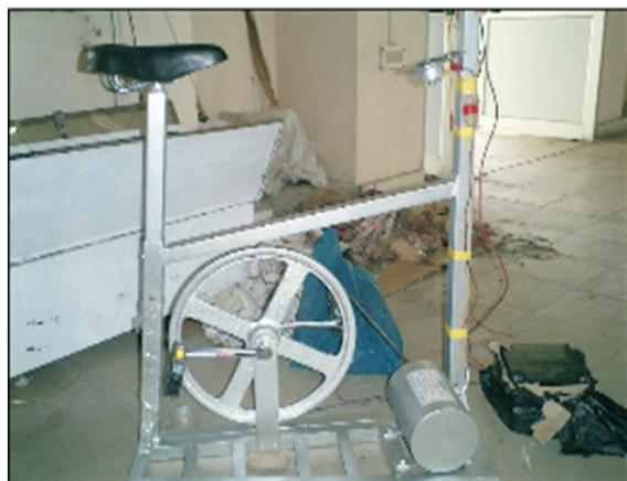
**Figure 3: Pedal operated power Generator**
